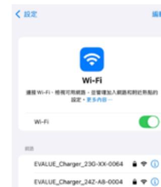
(4) When connected After connecting to WiFi, open a web browser and enter the charging station's ethernet IP address to access the charging station system webpage.
